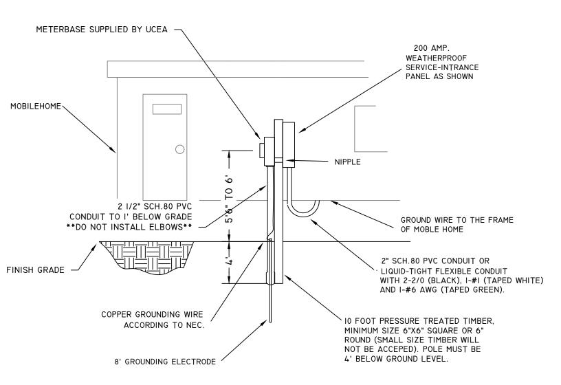
NOTE: ALL WIRING MUST COMPLY WITH THE STATE AND NATIONAL ELECTRICAL CODES
