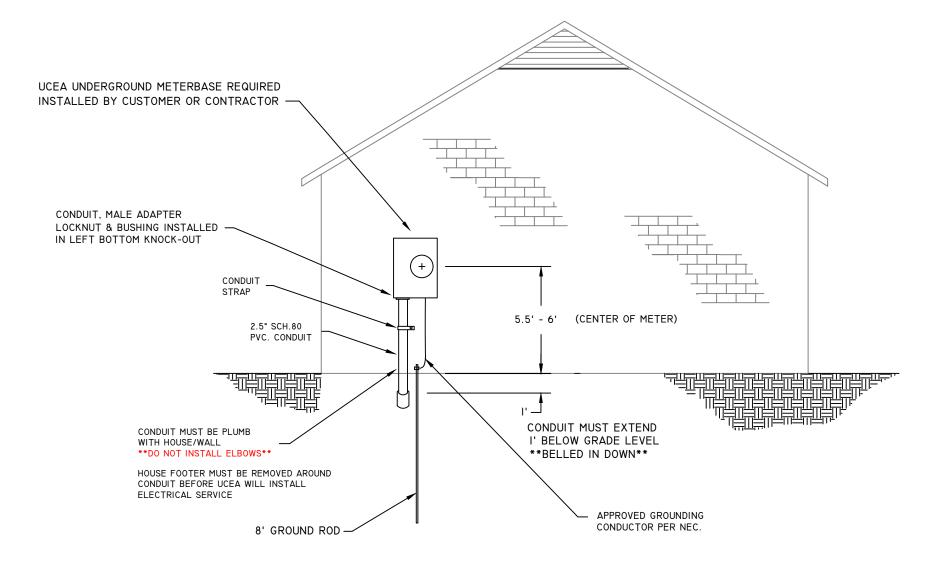
NOTE: ALL WIRING MUST COMPLY WITH ALL LOCAL, STATE, AND NATIONAL ELECTRICAL CODES -PANEL INSIDE HOUSE SHALL BE WITHIN 2 FT OF BACK OF METERBASE -METER LOCATION MUST BE APPROVED BY A EMPLOYEE OF UCEA
