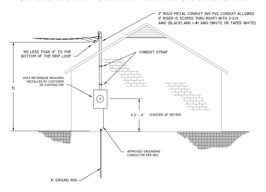
NOTE: ALL WIRING MUST COMPLY WITH ALL LOCAL, STATE, AND NATIONAL ELECTRICAL CODES -PANEL INSIDE HOUSE SHALL BE WITHIN 2FT OF BACK OF METERBASE
