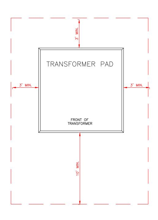
NOTE: THESE CLEARANCES ARE UCES MINIMUMS. GREATER CLEARANCES MAY BE REQUIRED BY CODES, DUE TO BUILDING CONSTRUCTION, TYPE OF TRANFORMER, LOCATION OF DOORS AND WINDOWS, ETC. CONSULT WITH UCEA.
